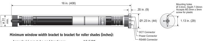
Acmeda 44mm tube and hardware 18 5/8" RollEase® 1.5" tube w/ Skyline Hardware 19 5/8" RollEase® 1.5" tube w/ R8 Hardware 18 1/2"
