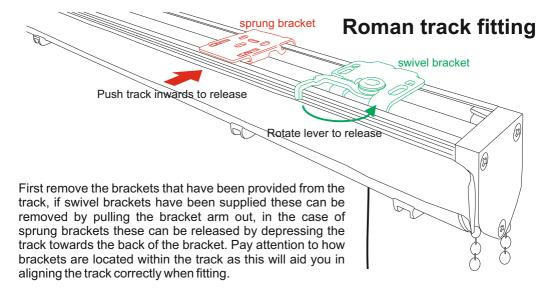
The correct number of fixing brackets for your track width will have been supplied and should be spaced approximately 8 cm in from each end, with the remaining brackets spaced evenly between them. Determine in which position the brackets will be fixed, either top or face, and then hold a bracket in position and mark the location of the two screws, repeat for each bracket. Drill screw holes and fit wall plugs if necessary, then screw each bracket into place.
